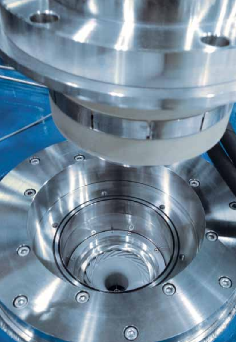
To achieve high efficiency and flexibility in Fermilab's new coldbox (far right), Linde Kryotechnik implemented a serial configuration of three cold compressors (above).
