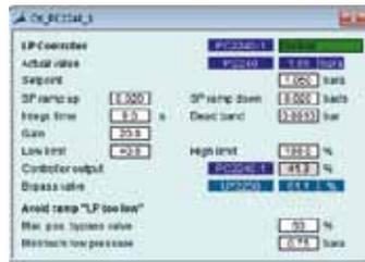
Controller pop-ups are opened directly with a click on the controller TAGs. The current control loop status is displayed and control settings can be modified. Control valve pop-ups allow switching between automatic or manual mode for positioning.
