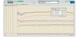
Data trends are sampled in live mode. Automatic data recording and backups ensure the availability of long-term records. The user can customise the display by adding or removing TAGs (identification labels of instruments and equipment), modifying curves or changing time settings.
