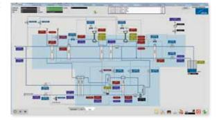
The schematic overview illustrates your plant as a process flow diagram. Different kinds of overviews are available to represent the plant in its actual operation modes and states. Process parameters, instrument values, warnings, alarms and other relevant data can instantly be observed.
